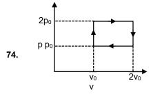
The above p-v diagram represents the thermodynamic cycle of an engine, operating with an ideal monoatomic gas. The amount of heat, extracted from the source in a single cycle, is :
